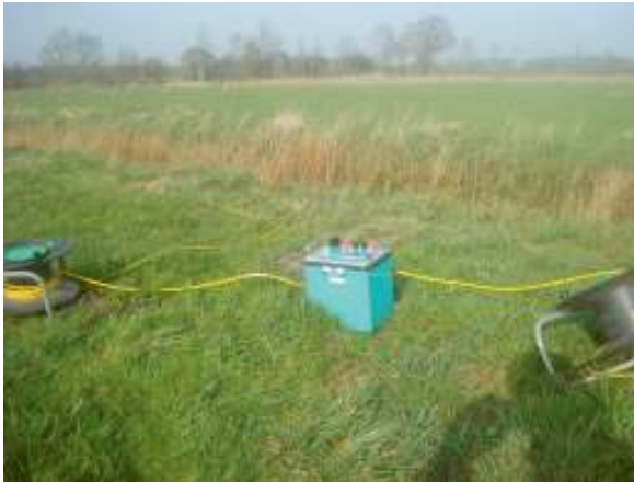
Figure 5.2: Photo of ERT measurements along ditch one
